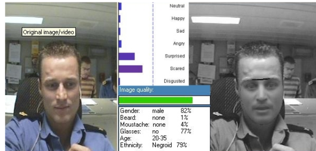
Fig. 5. Classification by the FaceReader [17] with a “below screen model”. Using a default model for the camera position decreases image quality and makes classification impossible.
