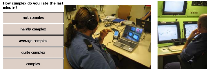
Fig. 3. Operator scoring complexity and effort during video replay of the just performed scenario (left and middle). Measuring pupil dilation (right).
